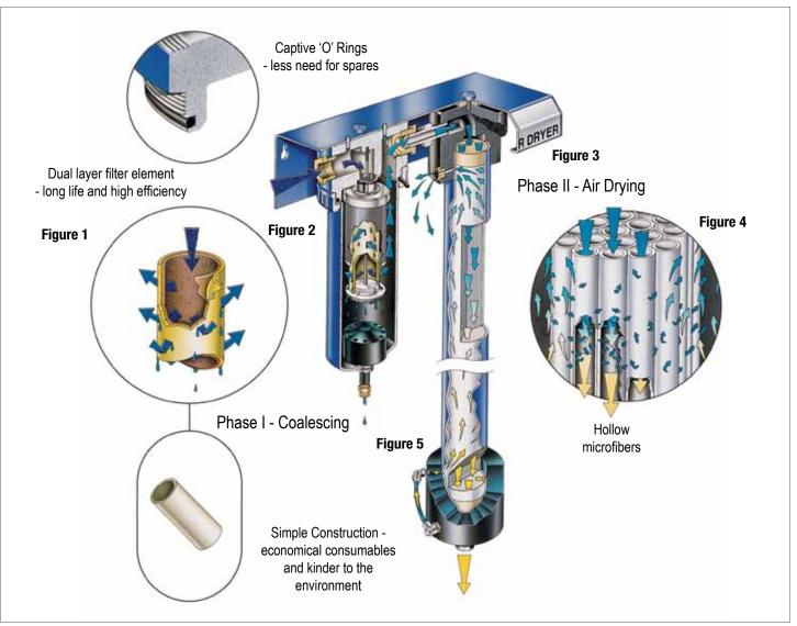
**Membrane Air Dryer - Principal of Operation**
